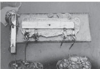
The first integrated circuit, a phase-shift oscillator, invented by Jack S. Kilby in 1958. (Courtesy of Texas Instruments.)
